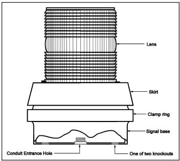
Figure 1. Catalog Series 51 Flashing Light with Horn
