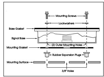
Figure 2. Direct Surface Mounting
