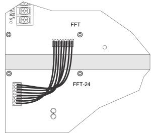
Figure 2 Wire Harness Connection
