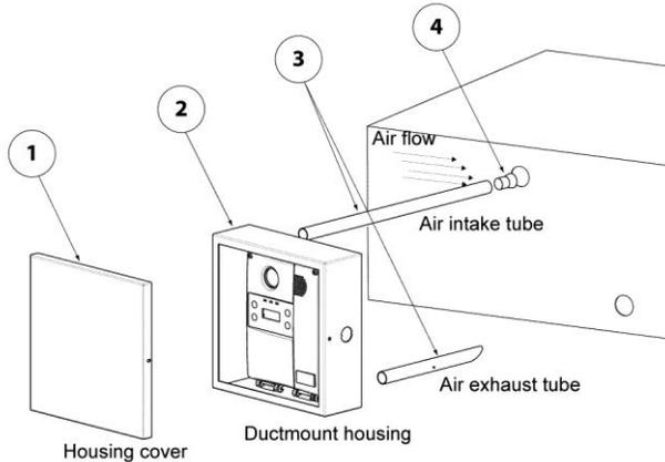
**Figure 2. Duct Mounting**
