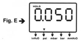
Press momentarily, DIF appears on top of the LCD and the display indicates the relative zero (relative zero causes the value of the display to show as "0.0") - only the amount of pressure change will be indicated. Press momentarily again and the unit returns to the normal mode of pressure differential (see Fig. F).
