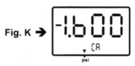
7. Again save the calibration point by pressing key, "SA" and "CA" appears in 2 seconds and then pressing "End" and "CA" appears in another 2 seconds. The meter turns back to the normal mode (see Fig. L).
