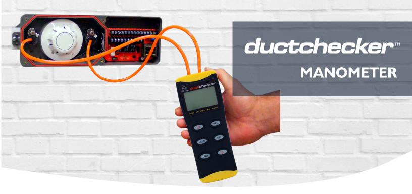
Duct Checker is the ideal device for annual testing to ensure that the duct detector will sample the airstream properly, as required by NFPA 72, and according to manufacturer's instructions.
