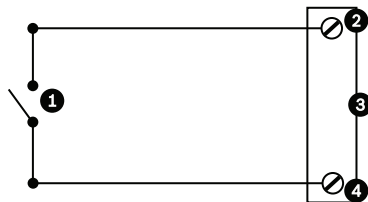
Figure 4.3 N.O. - Normally Open Non-supervised Connections
