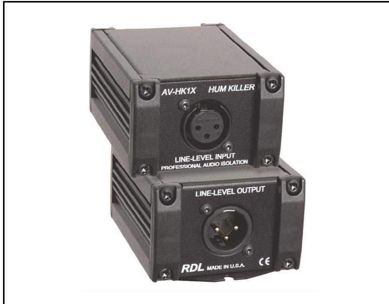
**APPLICATION:** The AV-HK1X is a mono transformer isolation module for use with a balanced, low impedance source and either a low or high impedance load. Input and output connections are provided on XLR jacks with gold-plated contacts.
