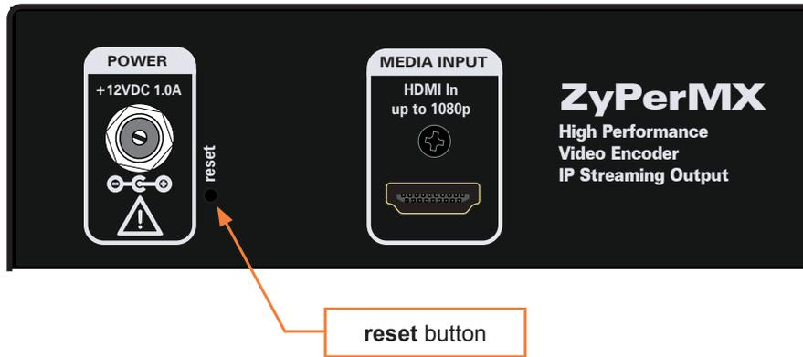
2. Press and hold the reset button, using the end of a paperclip or other pointed object. Wait approximately 5-10 seconds, then release the button.
