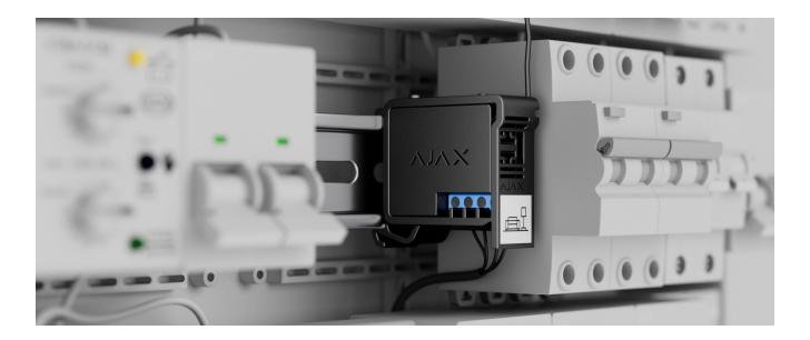
A  $39 \times 33 \times 18$  mm device is connected to the circuit gap. Relay dimensions allow installing the device into the deep junction box, inside the electrical appliance enclosure, or in the distribution board. A flexible external antenna ensures stable communication. To install Relay on a DIN rail, we recommend using a **DIN Holder**.
