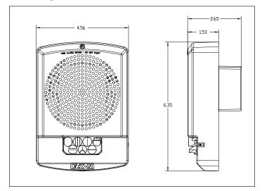
Figure 1. Wall Low Frequency Sounder Strobe
