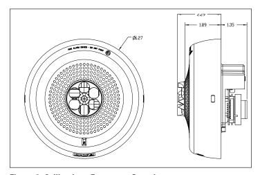
Figure 2. Ceiling Low Frequency Sounder
