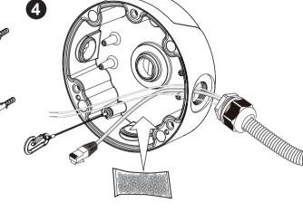
Attach a desiccant bag to the inside of the box. Note that the installation should be completed within 30 minutes so that desiccant remains effective.
