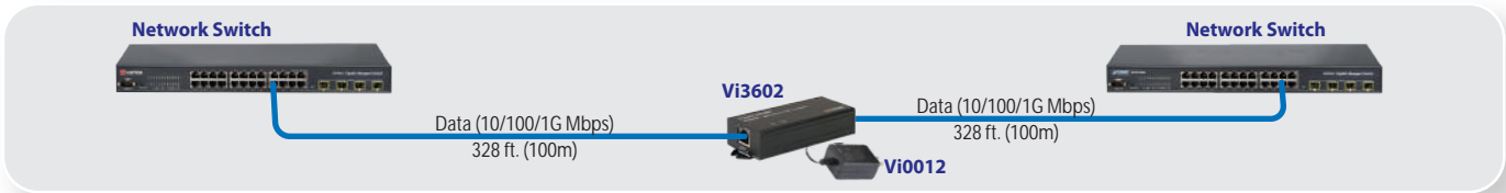
The Vi3602 can connect 2 network switches at distances up to 656 feet (200m) at 1000Mbps.
