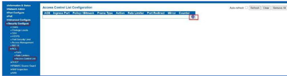
Figure 7-8-3 Access Control Limiters Configuration Screen
