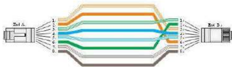
Figure 21: Crossover Wiring 1000Base-T Pin Assignments
