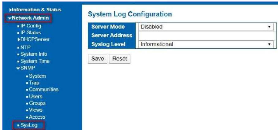
Figure 3-5 System Log Configuration Screen
