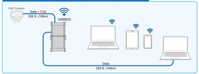
The Vi00023 has a built in switch that makes it possible to connect the IP camera to a network of wired and wireless devices.
