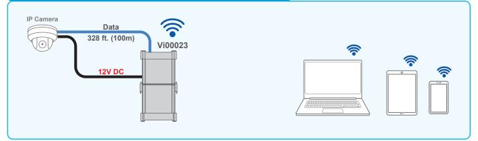
The Vi00023 enables connecting the non PoE cameras to any wireless device using a WiFi connection.
