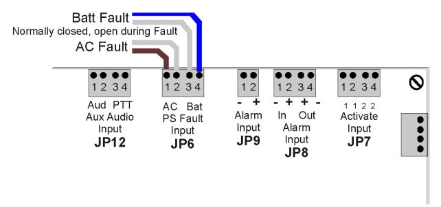
If the AC Supply monitoring function in not used, terminals 1 and 2 on **JP6** <u>must</u> be connected together using a jumper. Similarly, terminals 3 and 4 <u>must</u> be jumped if the power supply is not being monitored.
