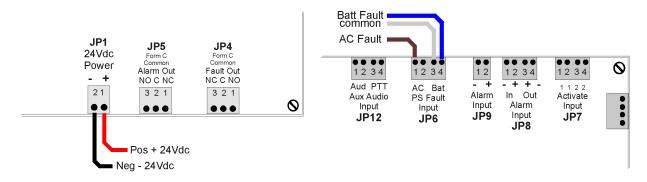
The external power supply's Fault / Trouble Normally Closed contacts should be wired to the JP6 connector on the VECP-25/50. This provides signaling to the VECP-25/50 that the AC is lost, and the system should go to its low-power battery-backup mode. This provides much more backup time during the AC fault, reducing the need for large batteries.
