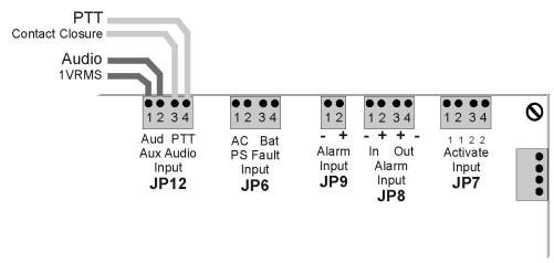
The VECP-25/50 is factory adjusted for an optimum signal level of 1Vrms on the audio input of **JP12**. The audio signal source must be adjusted to the appropriate level to ensure correct output volume and to avoid distortion. If it is not possible to provide a 1Vrms level, please consult the factory for information on how to adjust the system gain accordingly.
