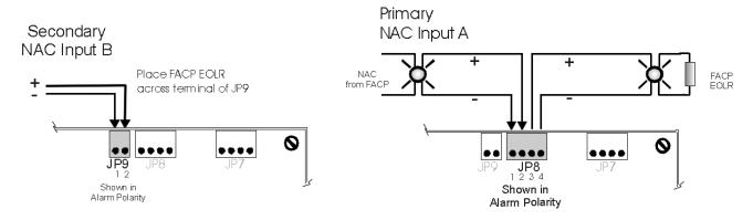
This wiring is supervised by the fire alarm control panel (FACP). It is power limited provided the FACP Bell Circuit is power limited
