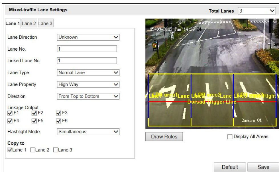
Figure 11-2 Mixed-Traffic Lane Configuration
