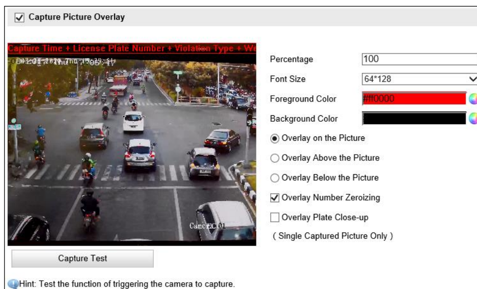
Figure 8-1 Single Picture Overlay
