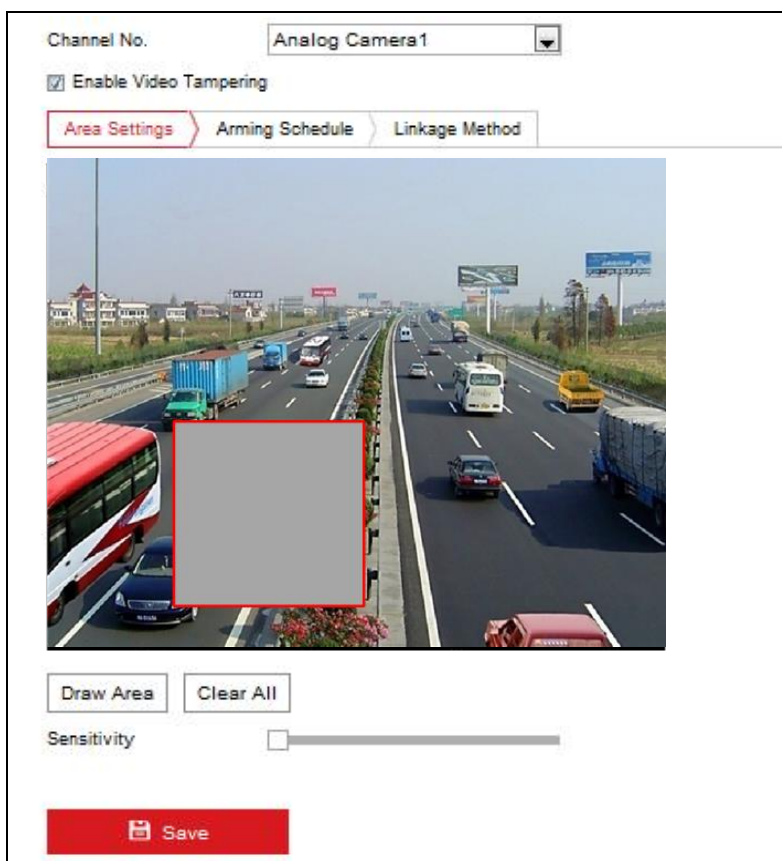
Figure 7. 15 Video Tampering Alarm Settings
