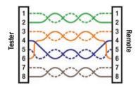
T568B is electrically identical to T568A but swaps the green and orange pairs. Either standard will work as long as the same standard is used at both ends of a run or patch cable. Mixing "A" and "B" creates a cross-over cable.
