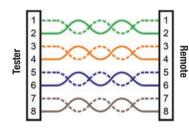
A common error in building a cable is to put all the pairs in pin sequence 1-2, 3-4, 5-6 and 7-8. This will produce the correct continuity, but the pairs are designated to be on pins 3-6and 4-5 in the middle of the connector for compatibility with phone wiring. This wiring error is only detected by the split pair test since the designated pairs are not twisted together.
