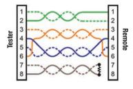
1 and 2 pins on the MapMaster mini are connected to pins 2 and 1 at the remote-end. The pins with this error are flashing. The "U" for the remote pin numbers indicates an unrecognizable continuity was detected that is neither a short or open. An ID remote connected to the MapMaster mini when in cable test mode would also show this error.
