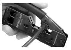
Grounding can be done using foil, braid, or a drain wire. Use the rear cavity of the Tele-Titan XG 2.0 to crimp external ground tab onto cable, securing the ground.
