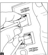
10) To Re-Open SnapJack: Using a small slotted screwdriver, lightly pry open the two EZ-Snap-Jack clasps (Fig 10).
