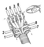
6 Flip the wire tray upside down and insert it into the connector pressing it firmly into place.
