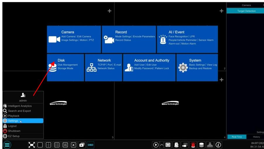
The setup panel includes seven modules. Each module provides some function entries with links for convenient operation. Here we take **Camera** module as an example. The **Camera** module provides convenient links such as “Add Camera”, “Edit Camera”, “Image Settings”, “Motion”, “IntelligenceAnalysis” and “PTZ”. Click **Camera** to go to the camera management interface as shown below.
