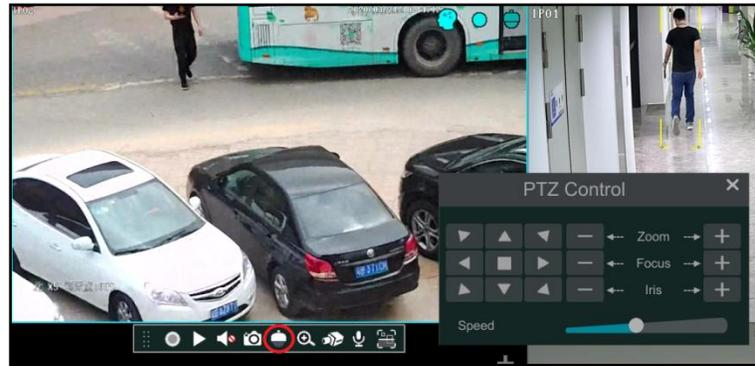
The direction, zoom, focus, iris and speed can be controlled in the small PTZ control window.
