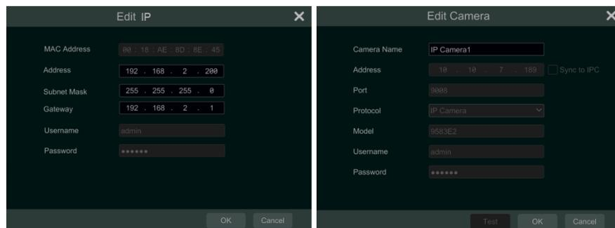
Click to edit the added camera as shown on the above right. Enter the new camera name, IP address, port, username and the password of the camera. You can click “Test” to test the effectiveness of the input information. Click “OK” to save the settings. You can change the IP camera name only when the added camera is online. Click “Next” to continue.
