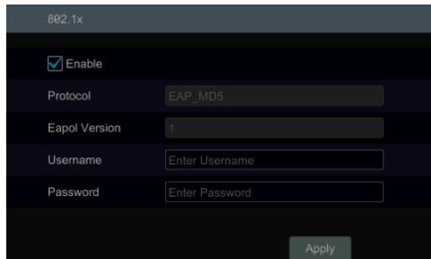
To use this function, the NVR shall be connected to a switch supporting 802.1x protocol. The switch can be considered as an authentication system to identify the device in a local network. If the NVR connected to the network interface of the switch has passed the authentication of the switch, it can be accessed via the local network.
