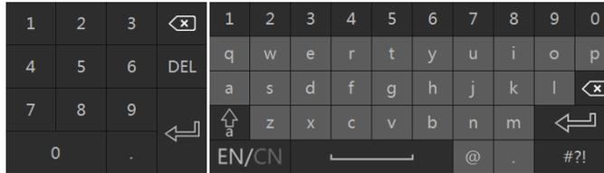
The system includes two input boxes. Refer to the above pictures. The left box is the number input box and the right box is the input box which provides inputs of numbers, letters and punctuation characters. The introductions of keys on the input boxes are shown below.
