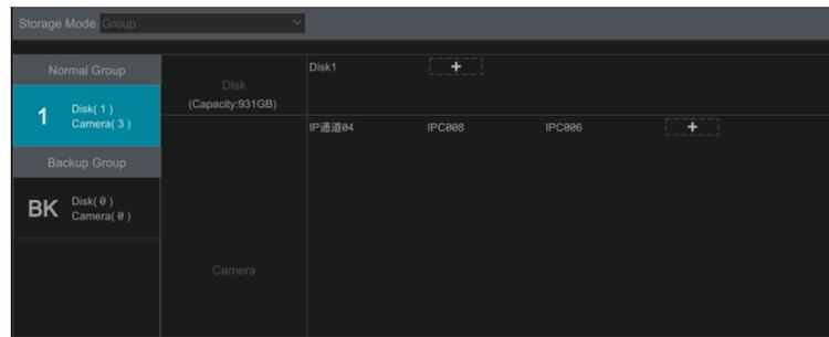
There are all two disk groups. By using disk group, you can correspond the camera to disk (the record data of the camera in the group will be stored into the disks in the same group). The NVR with e-SATA interface supports e-SATA recording.
