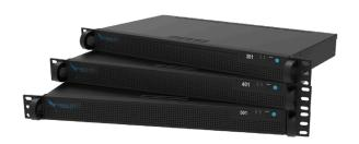
The Bridge acts as a gateway from your premises to the Cloud Data Center where your video is stored and managed by the Cloud Cloud VMS. It provides video buffering, a secure connection, bandwidth management, and monitoring of cameras.
