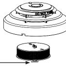
Pry the **elastic arm** gently with a small, slotted screwdriver to remove cage for cleaning.
