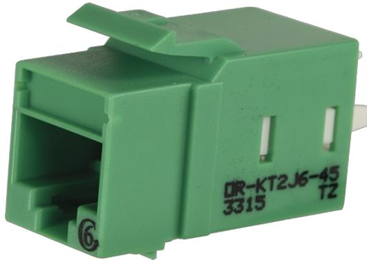
Category 6 Keystone jack, 8-position, 180 degree exit, icon compatible, T568A/B wiring, Green , individually packaged. Keystone, KT2J jacks and modules feature New installer friendly lacing cap termination with free termination tool in every carton. The keystone footprint allows flexibility in installation scheduling because its rear insertion into the faceplate allows the technician to complete the termination before and during the construction process.
