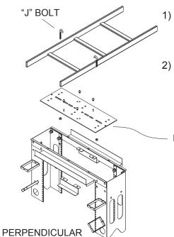
1) Attach the ladder mounting plates to the MK rack using the brackets and hardware as shown.
