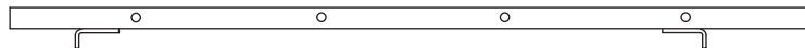
(Top view showing front rackrail installed in position 2, and rear rackrail installed in position 3)
