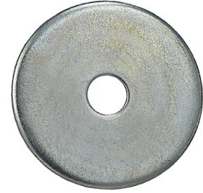
Fender Washers differ from standard Flat Washers in that their outside diameters are much larger in proportion to their center holes. With this design, a fender washer can be placed under the head of a bolt or nut, to help distribute forces applied when tightening, or to cover an oversized hole.
