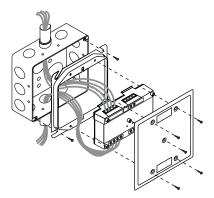
**GSA-MCC1S:** mount the UIOxR motherboard inside a suitable Kidde enclosure with screws and washers provided. Plug the module into any available position on the motherboard and secure the module to the motherboard with the captive screws. Wiring connections are made to the terminals on the motherboard (see wiring diagram). UIOxR motherboard terminals are suited for #12 to #18 AWG (2.5 mm² to 0.75 mm²) wire size.
