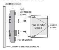
**GSA-MIO:** mount the UIOxR motherboard inside a suitable Kidde enclosure with screws and washers provided. Plug the module into any available position on the motherboard and secure the module to the motherboard with the captive screws. Wiring connections are made to the terminals on the motherboard (see wiring diagram). UIOxR motherboard terminals are suited for #12 to #18 AWG (2.5 mm² to 0.75 mm²) wire size.
