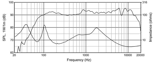
Half-space (2pi, mounted in ceiling); input impedance (lower solid line)
