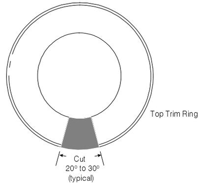
Slide the ring through the ceiling cutout, as shown, and place it in position above the ceiling surface.
