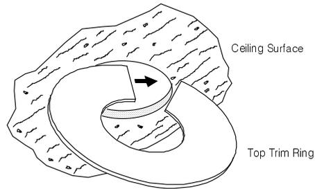
When possible, orient the speaker's mounting tabs so that all tabs tighten onto the top trim ring.
