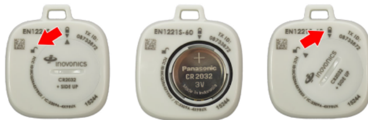
Figure 7 - SF503UL and SF504ES Battery Replacement
