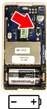
Figure 14 - SF502ES Battery Orientation
