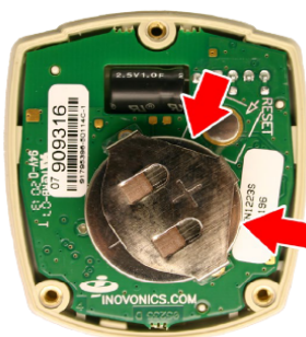
Figure 9 - SF501ES Battery Removal
