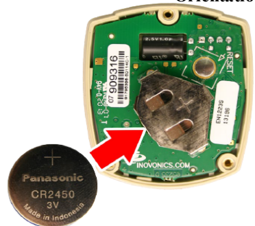
Figure 10 - SF501ES Battery Orientation
