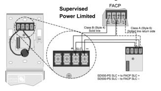
Figure 1: Fire Pull Station Wiring
