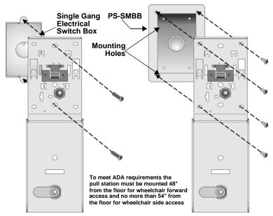
Figure 2: Mounting the Fire Pull Station
