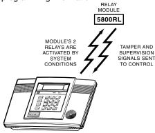
Figure 1. Lynx Interface Diagram
