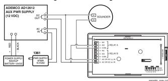
Figure 3. Typical Sounder Wiring Installation Setting Up the 5800RL
