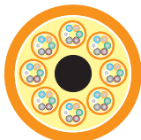
48-fibers (8 tubes of 6-fibers)
