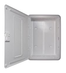
Constructed with a robust, wireless transparent ABS plastic material, this lightweight, low-profile enclosure is designed to integrate wireless devices into traditional structured wiring installations. , The enclosure mounts easily for both surface and recessed applications, and the hinged door is equiped with extra venting along the vertical plane for superior heat disipation.
