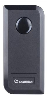
GV-SR1352 is a dual-band RFID card reader that recognizes access control cards. Featured with Wiegand outputs, GV-SR1352 can be connected to any Wiegand-compatible access control systems. Its dual-band capability offers great flexibility for integrators to solve card management issues on the locations, installed with both 125 kHz and 13.56 MHz readers. For outdoor use, GV-SR1352 comes with a weather-sealed and IP66-compliant housing.
