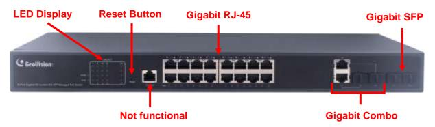
**IMPORTANT:** The 2 SFP ports labeled 17S ~ 18S are associated with the 2 RJ-45 ports labeled 17T ~ 18T respectively. When one of the two associated ports is used, the other port will not work. For example, if the Gigabit SFP port labeled 17S is used, the Gigabit RJ-45 port labeled 17T will not function.
