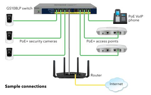
This switch is designed for indoor use only. If you want to connect it to a device located outdoors, the outdoor device must be properly grounded and surge protected, and you must install an Ethernet surge protector inline between the switch and the outdoor device. Failure to do so can damage the switch.
