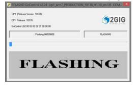
12 After status bar completes on the first "Flashing" screen, the second "Flashing" screen appears:
