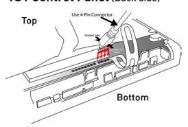
WARNING: When inserting the Firmware Update Cable (with the extender pins) it is EXTREMELY IMPORTANT to insert the cable with the flat side DOWN and the slotted side UP.
