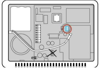
**IMPORTANT:** Make sure that the slotted side of the connector is facing away from the tab on the J4 connector. Failure to do so may result in damage to the Control Panel.
