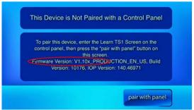
Make sure that the Firmware Version on the Control Panel matches the Firmware Version on the TS1 before attempting to "learn-in" or pair the TS1 with the Control Panel.
