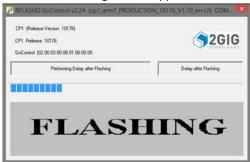
IMPORTANT: DO NOT disconnect the cable, the power to the Control Panel, or close the Firmware Update Tool until the status bar has completed and the final screen appears (showing the updated firmware version).
