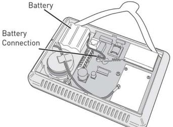
4 Disconnect the power supply from TB1 and 2 on the Control Panel terminal block or unplug the panel power supply from the wall outlet.
