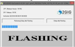
**IMPORTANT:** DO NOT disconnect the cable, the power to the TS1, or close the Firmware Update Tool until the status bar has completed and the final screen appears (showing the updated firmware version).
