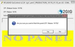
NOTE: If the screen displays a RED FAIL message, check to ensure that the firmware update cable is plugged into your PC correctly in the proper USB slot. Also check to ensure that the correct COM Port appears in the Firmware Update Tool Shortcut's Target field.
