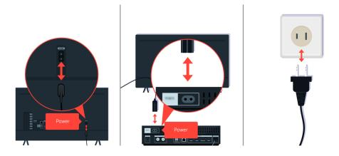
First disconnect and reconnect the power cables and HDMI cables on the back of your TV or the One Connect Box, then unplug the power cord and plug it back into the wall outlet.
