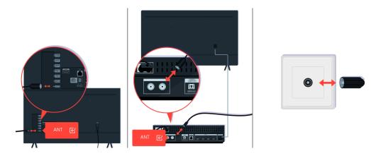
Check the antenna and input cable connections.
