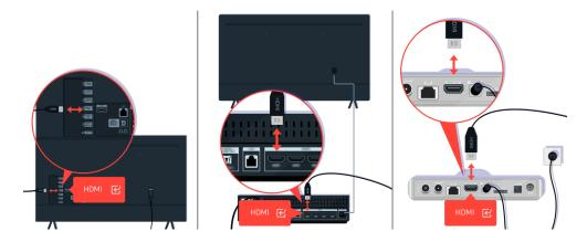
Check the antenna and HDMI cable connections.
