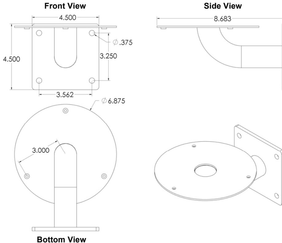
ETP-MBKT fits a 4" square box or a 1900 box and extends 8.75" from a wall. Tube is hollow to enable wires to run from ETP-EL into a conduit box.
