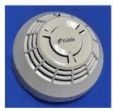
The KC2 Heat Detector is a conventional low-profile, self-diagnostic, two-wire detector which uses a dual rate-of-rise and fixed-temperature heat sensor to determine when to signal an Alarm condition. The rate-of-rise function quickly detects a fast, flaming fire. The fixed-temperature function detects fire when the air temperature near the detector exceeds the alarm point of 135 °F (nominal). When used
