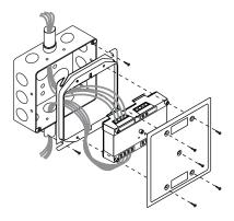
**GSA-MRM1:** mount the UIOxR motherboard inside a suitable Kidde enclosure with screws and washers provided. Plug the module into any available position on the motherboard and secure the module to the motherboard with the captive screws. Wiring connections are made to the terminals on the motherboard (see wiring diagram). UIOxR motherboard terminals are suited for #12 to #18 AWG (2.5 mm2 to 0.75 mm2) wire size.
