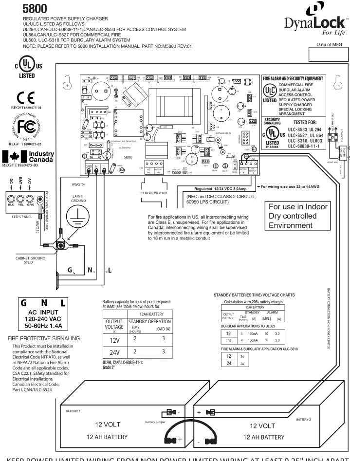
KEEP POWER LIMITED WIRING FROM NON POWER LIMITED WIRING AT LEAST 0.25" INCH APART
