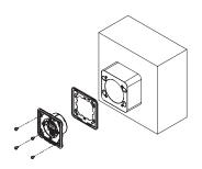
Insert the seal as shown on the surface-mounted box
