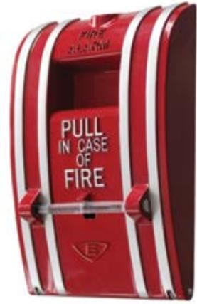
Edwards 270 Series non-coded single-action fire alarm stations are sturdy, attractive, and designed for economical installation. The station provides a single action, break glass, initiating operation. It is available with normally open (N.O.), normally closed (N.C.) or combination N.O./N.C. contacts. The 270 Series have screw terminals for field connection. The 270A Series Manual Stations have 6 inch (150mm) wire leads.
