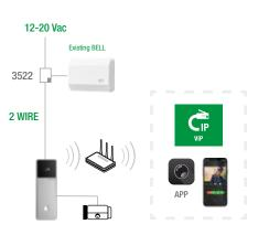
VISTO VIP WI-FI WITH EXISTING POWER SUPPLY AND CHIME
