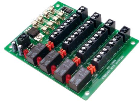
Door control relay modules ensure compatibility of access hardware components and simplify system installation and troubleshooting. Modules may be ordered with or without power supplies. Different modules may be specified for one power supply. The isolated relay design allows small gauge cable runs of 22 gauge wire up to 1000 feet from the trigger device to the module.
